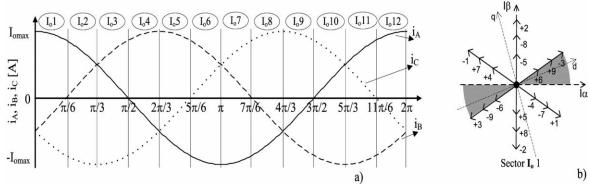
Figure 5: (a) Output Currents and their Corresponding Sector. (b) Input Current State-Space Vectors, when Output Currents a Relocated at Sector  $I_01$ . The dq Axis is Represented, Considering that the Input Voltages are Located in Zone  $V_i1$
