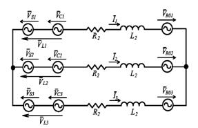
Figure 2: Three Phase Equivalent Circuit of the Matrix UPFC and Transmission Line
