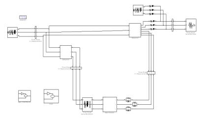
Figure 7: Transmission Network with Matrix Converter – UPFC
