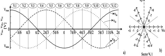
Figure 4: (a) Input Voltages and their Corresponding Sector. (b)Output Voltage State Space Vectors when the Input Voltages a Relocated at Sector  $V_i \mathbf{1}$
