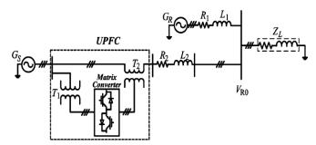
Figure 1: Transmission Network with Matrix Converter UPFC
