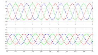
Figure 12: Line Currents  $(i_A, i_B, i_C)$  and Input Matrix Converter Currents  $(i_a, i_b, i_c)$  pu
