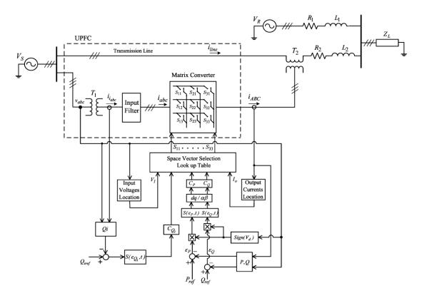
Figure 6: Control Scheme of Direct Power Control of the Three-Phase Matrix Converter Operating as a UPFC
