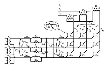
Figure 3: Transmission Network with Matrix Converter UPFC
