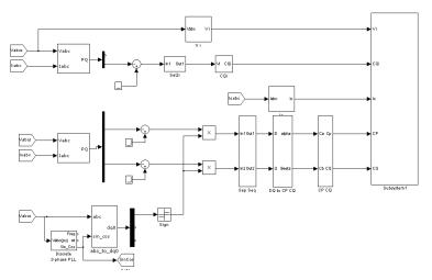
Figure 8: Control Scheme of Matrix Converter as UPFC Using Space Vector Selection Table
